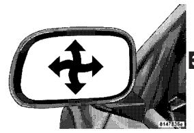
To adjust a mirror, turn the control wand toward the left or right mirror positions indicated. Tilt the control wand in the direction you want the mirror to move. When finished adjusting the mirror, turn the control to the center position to prevent accidentally moving a mirror.
